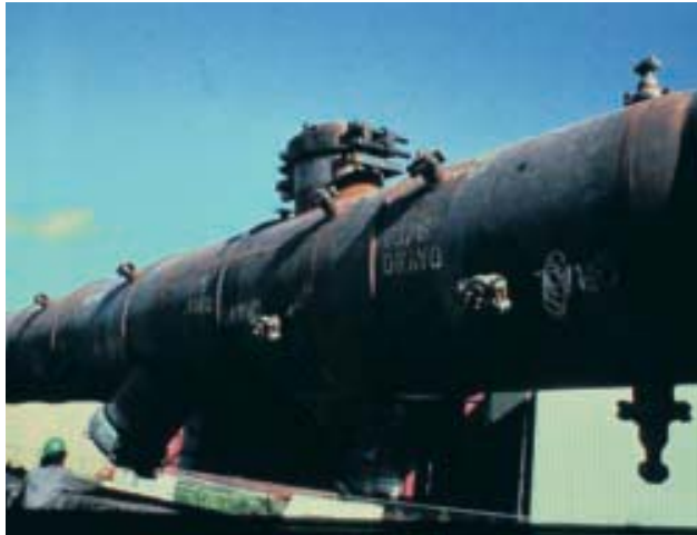
The Office of Coal Research, U.S. Department of the Interior, and the American Gas Association jointly sponsored a program to develop coal gasification technology. On this pre-quench tower for raw gas purification, two Grayloc vessel closures and several smaller Grayloc connectors were used for pressures of 1,650 psi and temperatures to 650° F.
